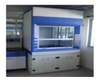
Chemical fume hoods, when used properly, are one of the most reliable engineering controls in the laboratory. They protect workers by: Containing vapors, dusts, gases, and fumes generated within the hood, and removing them as air flows into the hood and then out via the laboratory exhaust system.
