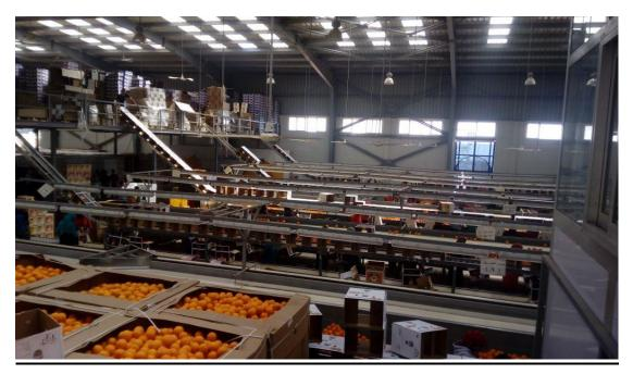
The packing process is preceded by the sizing process, which is made by the sizing machine, Sizer, which distributes the fruits according to sizes in its appropriate packing basin.
