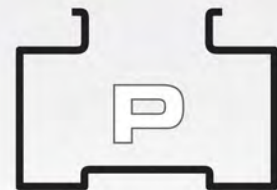
Made in three versions, with 1.5 mm, 2.0 mm and 2.5 mm thick steel.
